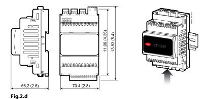
Apply slight pressure to the controller resting on the DIN rail until the rear tab clicks into place.
