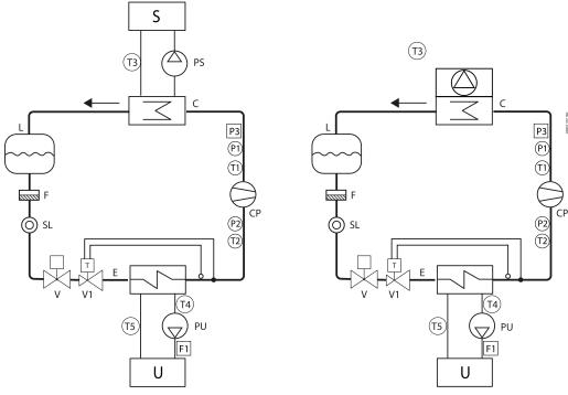
Fig.2.r: water-cooled unit (left) and air-cooled unit (right)
