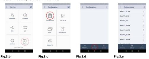
4. apply the selected configuration via NFC or Bluetooth. The refrigerant has now been correctly configured;
